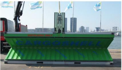
container constructed with a polymer shell and steel frame could be broken down, the shell ground into plastic pellets (the form needed for molding) and the pieces of several containers transported in a single box."
